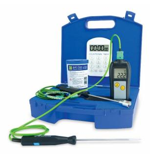
The Legionnaires thermometer kit is specifically designed for legionnella testing and can be used to monitor the temperature of both standing water and the surface of pipes and tanks that form part of the water system.
