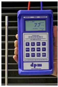
The TT 570 Low Res Micromanometer with its unique differential capacitance transducers and programmable auto zero facility stores a maximum of 2500 readings.
