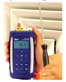
Digital Pocket Manometer allows the engineer to select velocity resolution.
